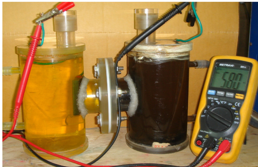
Fig. 1. Schematic details and photograph of dual chambered MFC used in the experiments.
